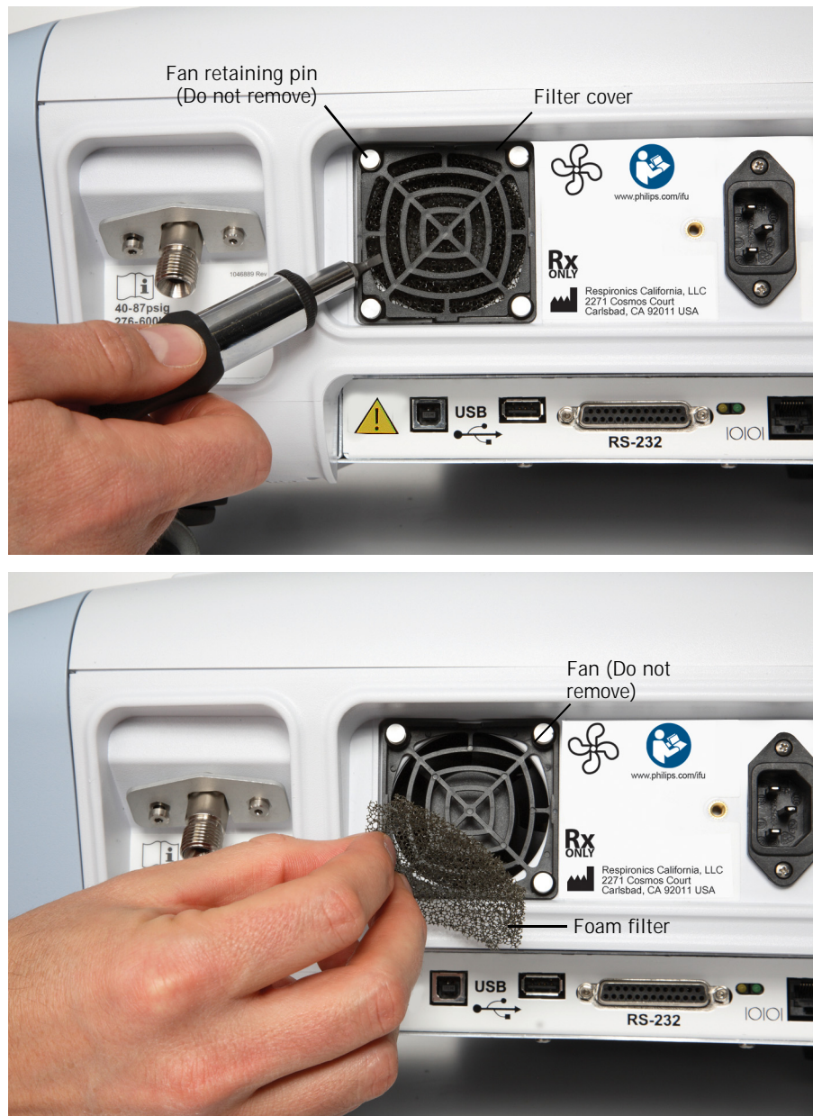
Figure 10-2: Replacing the cooling fan filter
